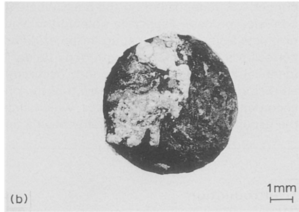
Figure 2 The screw after explantation: (a) total view and (b) screw head
